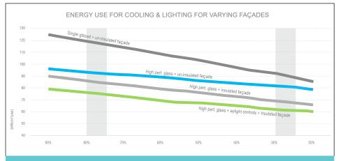
The linear relationship between WWR and energy consumption for the lighting and cooling of an office building in Manila in the Philippines as simulated using the EDGE App.
